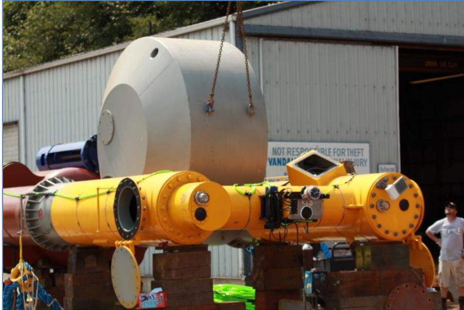
Figure 14 - Top View of PowerPod Showing the Dry Box
