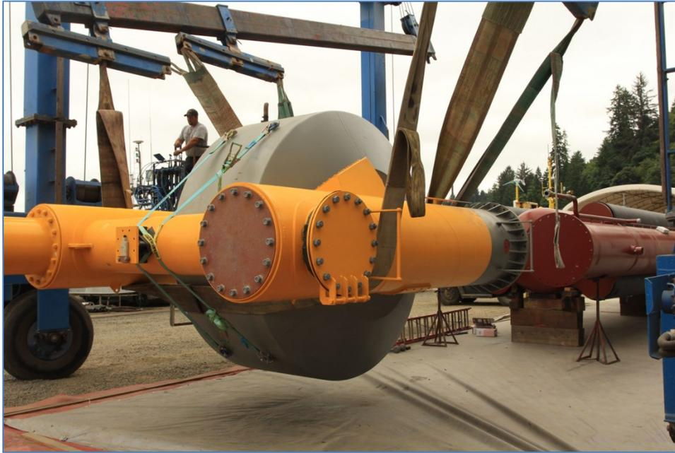
Figure 8 - PowerPod being mated to Hull prior to Oregon deployment. Float has subsequently been modified to teardrop shape.
