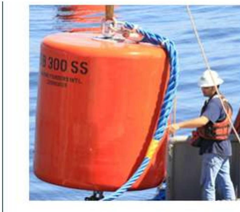
Figure 10. SB-300 Subsurface Float
