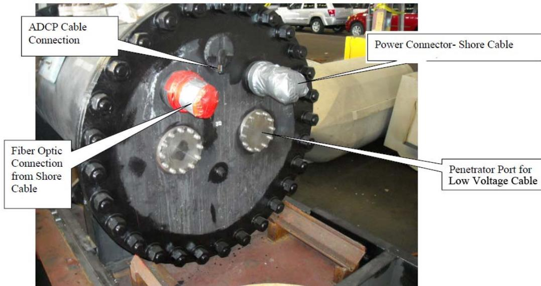
**Figure 29 – T-Pod End Cap with Connectors**
