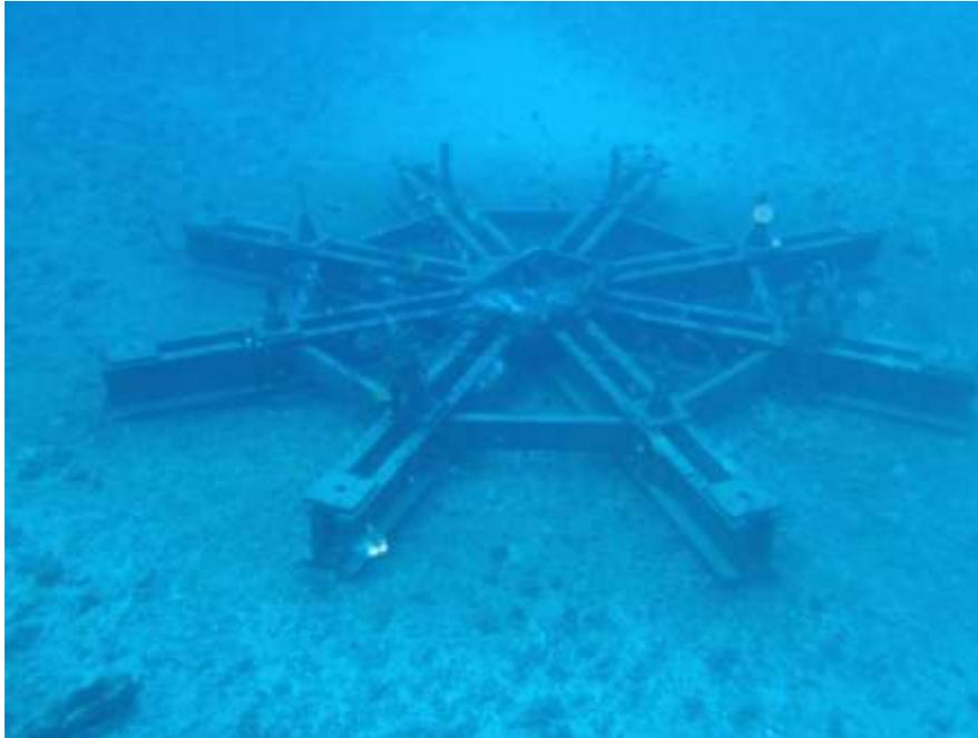
**Figure 6. WETS Rock Bolted Anchor Frame MC**
